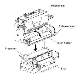
④ Fasten the presenter to the mechanism using the two screws.
